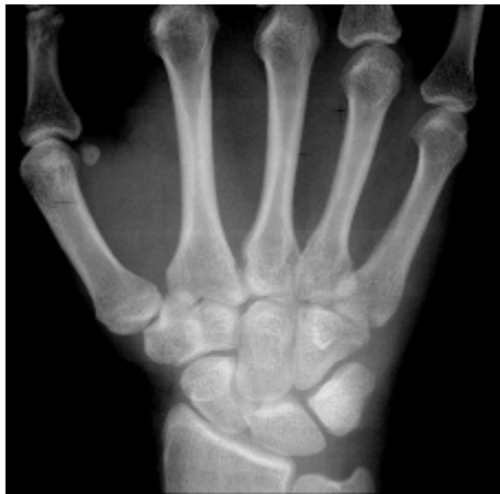
Image with a micro-focus X-ray generator of 5 µm and PIXRAY with a pitch of 50 µm.
