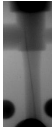
Crack detection in a 13 cm thick metal block.
